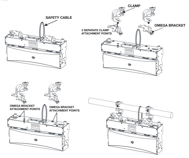
Screw one clamp each via a M12 screw and nut into the Omega bracket. Insert the quick-lock fasteners of the Omega holder's into the respective holes on the bottom of the Allegro Z6. Tighten the quick-lock fasteners fully clockwise. Pull the safety cable through the openings located on the base and over the trussing system or a safe fixation spot. Insert the end in the carabine and tighten the safety screw.
